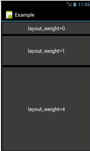
**FIGURE 2.8** A linear layout with three buttons demonstrating `layout_weight`
