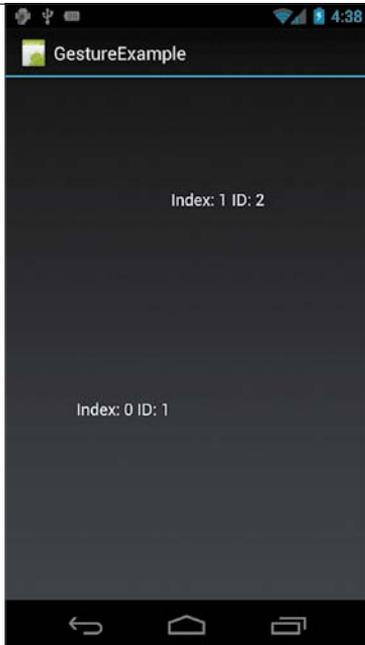
**FIGURE 8.2** The index and ID of each pointer will be displayed as you place your fingers on the screen.
